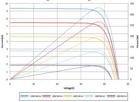
Excellent performance under weak light conditions: at an irradiation intensity of 200 W/m<sup>2</sup> (AM 1.5, 25 °C), **96.5%** or higher of the STC efficiency (1000 W/m<sup>2</sup>) is achieved
